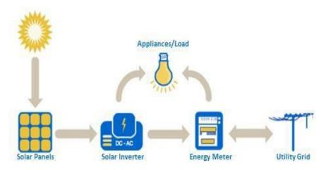
Main components of a Grid Connected Rooftop Solar PV system:
