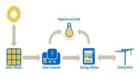
Main components of a Grid Connected Rooftop Solar PV system:
